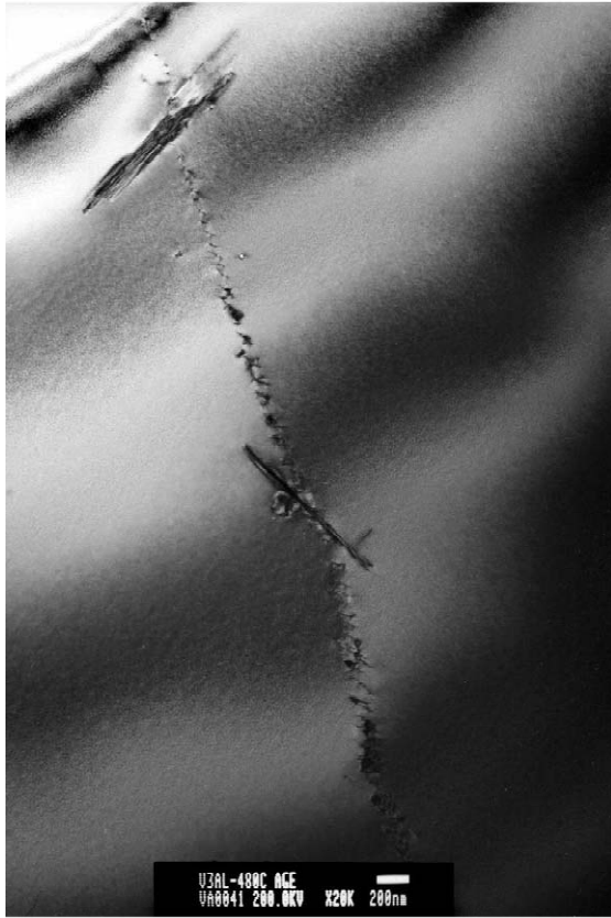
Fig. 7. TEM image of a sub-boundary of aged V–30Al.
